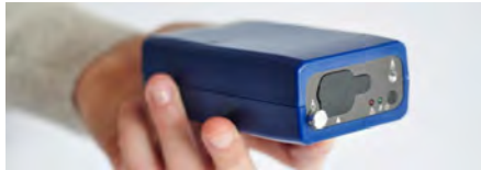
Fig. 7.2 Microaethalometer: device used as a reference for calibration.
